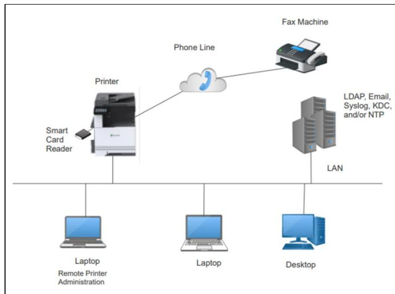
Figure 1: TOE Architecture
